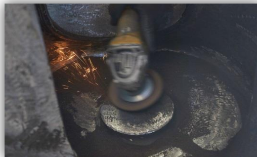
Surface grinding prep for a ductile iron casting
