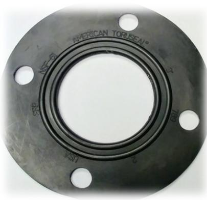
Clean flange faces and faced pipe ends thoroughly prior to installation. Do not use joint or gasket compounds with Toruseal® gaskets (assemble joints dry).
